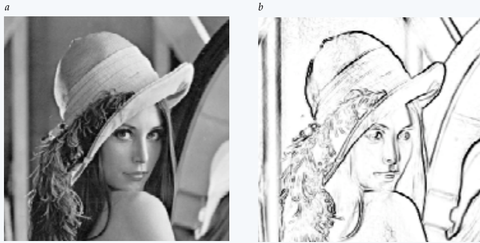
Figure 7. The original image of "Lena" (a) and its edges detected by a gradient related algorithm (b).
