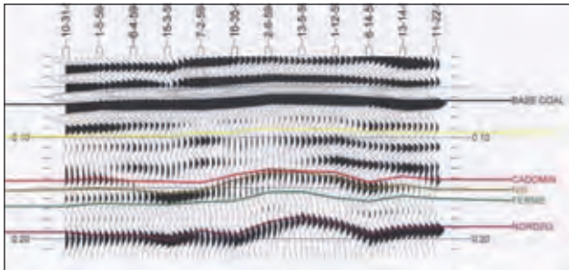
Figure 7 Conventional forward modelling yields no consistent porosity signature.
