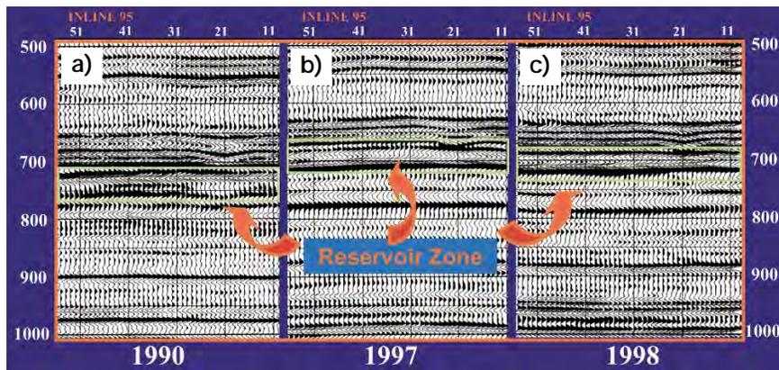
**Figure 6.** 4-D migrated stack sections before cross-equalization: (a) baseline in-line 95 from 1990 survey; (b) monitor in-line 95 from 1997 survey; and (c) monitoring in-line 95 from 1998 survey. Note phase variations, amplitude differences, and time shifts.
