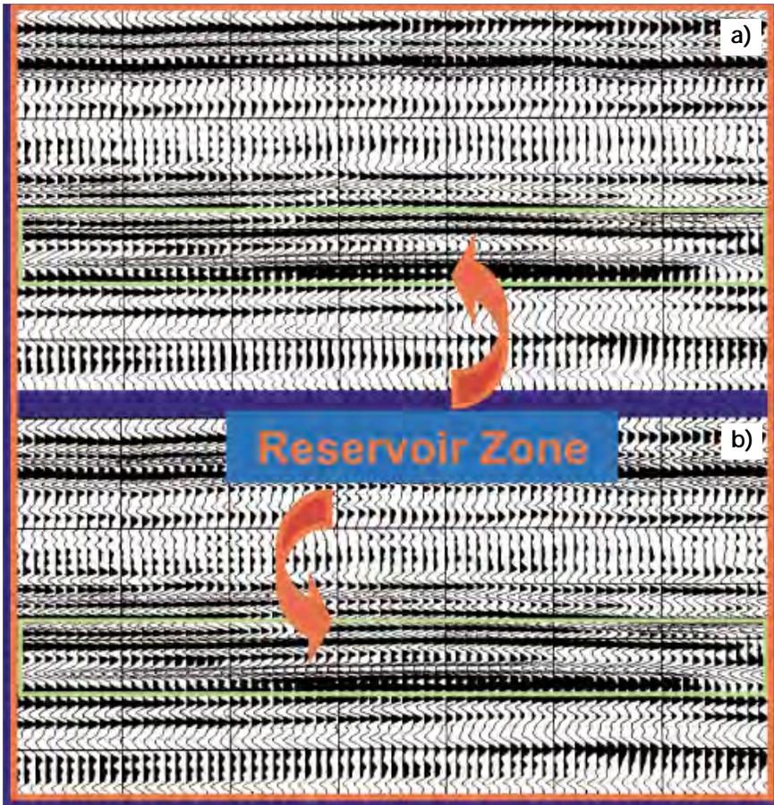
**Figure 5.** Effect of prestack amplitude balancing. Migrated stack sections (a) without and (b) with amplitude normalizations applied subsequent to prestack single-trace zero-phase spiking deconvolution following surface-consistent deconvolution.
