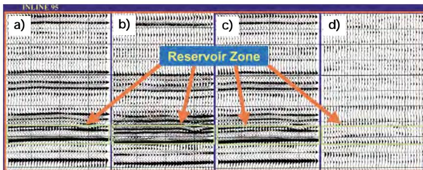
**Figure 8.** Cross-equalization results using a long design window (250-1350 ms). (a) In-line 95 of 1997 survey as reference; (b) in-line 95 of 1998 survey as input; (c) output of cross-equalization applied to (b); and (d) difference of (a) and (c). Filter contains bandwidth normalization, rms energy, phase matching, and time correction.
