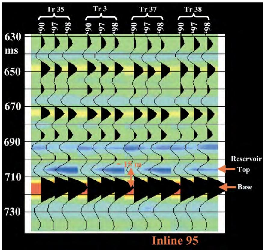
Figure 10. Time lapse trace-to-trace comparison, illustrating the effect of steam heating on seismic signatures.
