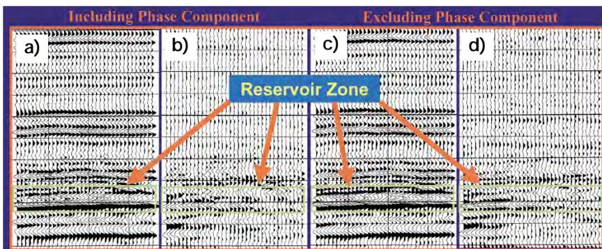
**Figure 9.** Cross-equalization results using a short design window (200-600 ms). (a) Filtered in-line 95 section; (b) Difference between (a) and Figure 8a; (c) Filtered section using an operator excluding the phase-matching component; and (d) difference between (c) and Figure 8a.
