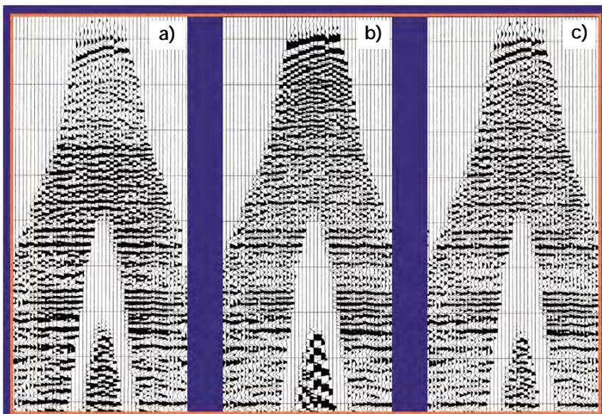
Figure 4. Prestack amplitude balancing. Shot record (a) after surface-consistent deconvolution and single-trace zero-phase spiking deconvolution; (b) after adding amplitude rescaling to (a); and (c) after adding a global scale correction to (c).
