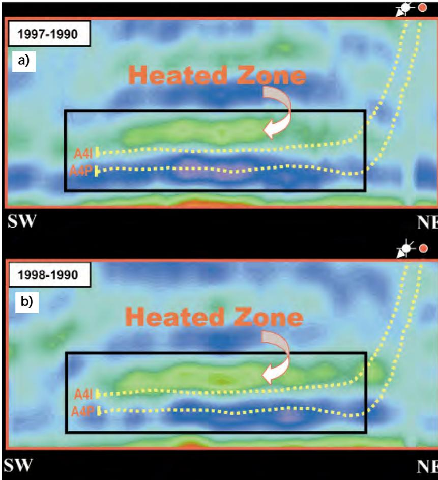
Figure 13. 4-D seismic difference section. Highlighted zone shows that the steam chamber is expanded along horizontal well pair A4. (a) Difference between 1997 and 1990 surveys and (b) difference between 1998 and 1990 surveys.
