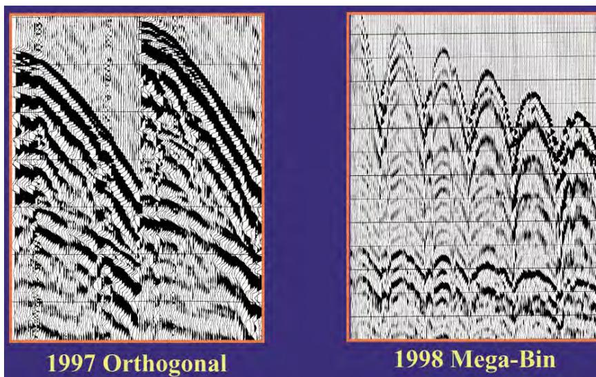
**Figure 2. Raw shot records from 1997 (left) and 1998 monitoring surveys.**
