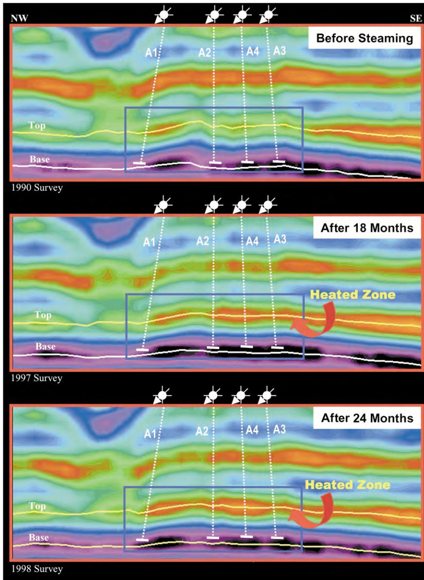
**Figure 11. Steam chamber developing across the pattern of four SAGD horizontal wells.**
