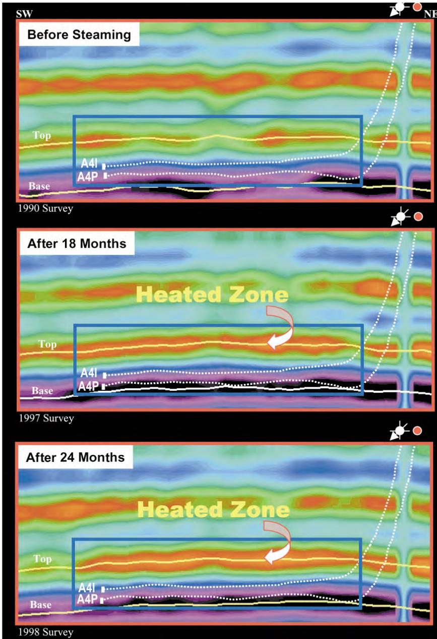
**Figure 12. Steam chamber developing along horizontal well pair A4.**
