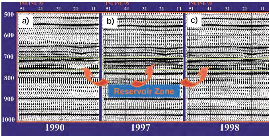
**Figure 7.** 4-D migrated stack sections after cross-equalization. The filter operator was designed from a time window of 250-2350 ms. Input data to filter are in Figure 6. (a) Baseline 1990 section as reference; (b) monitoring 1997 section; and (c) monitoring 1998 section. Filter contains bandwidth normalization, rms energy balancing, phase matching, and time correction.
