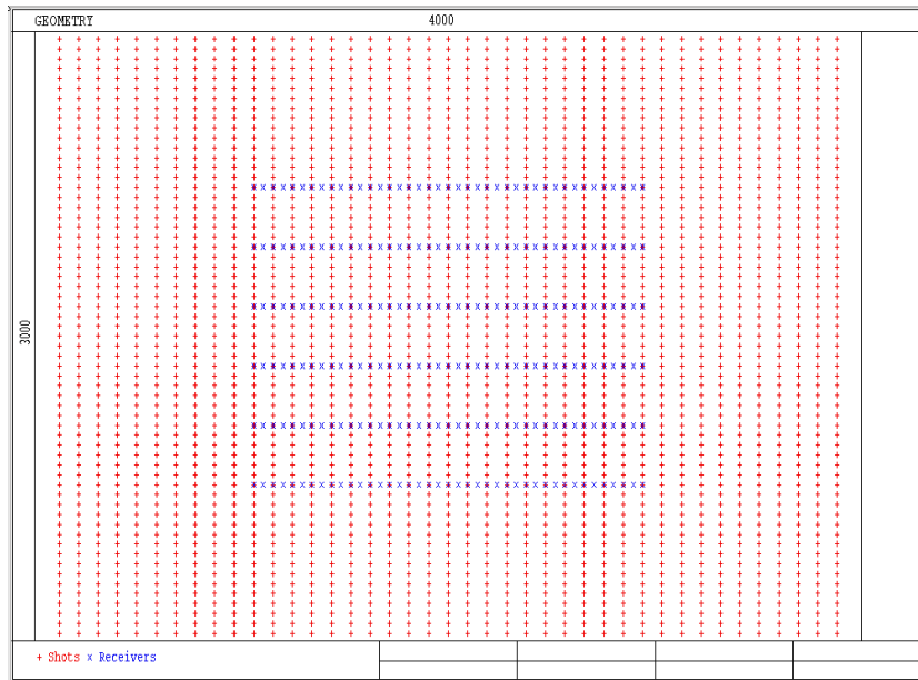
Figure 6. Source and receiver geometry for 3C-3D design example 2. Shot line spacing is 100m, receiver line spacing is 300m and shot and receiver spacings are both 50 m.
